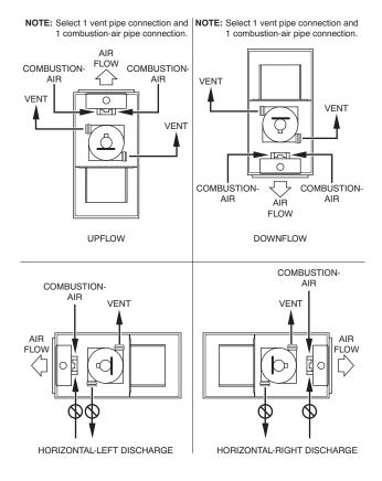
Fig. 36—Combustion-Air and Vent Pipe Connections
